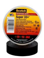
Scotch® Super 33+ Vinyl Electrical Tape is a 7 mil thick, premium grade tape that provides electrical insulation for all wires and cables rated up to 600V. The flame retardant tape withstands a temperature range of 0 to 221 °F ( 18 to 105 °C). It is compatible with solid dielectric cable insulation, synthetic cable insulations, jackets and splicing compounds.
