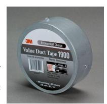
3M Value Duct Tape 1900 is a good toolbox tape for general applications including light-duty sealing, bundling, marking, and temporary repairs in non-critical applications. Its synthetic rubber adhesive sticks on contact to smooth metal, glass, plastic, sealed concrete and more, and the water-resistant polyethylene coating seals well in moist and humid environments.
