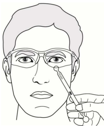
Figure 5B: Checking Gap
